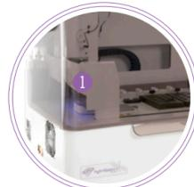
Adapted to DNA Flow technology, capable of holding 24 samples during the hybridisation process and 48 PCR tubes during the amplification process.
